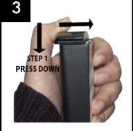
With the keypad facing away from you, close the cover by gently pressing it down (STEP 1) and sliding it until it aligns with the front (keypad) of the device (STEP 2).
