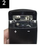
Install 2 AAA batteries. Make sure the + and symbols on the metal hinge of the battery compartment correspond with the + and - end of each battery.
